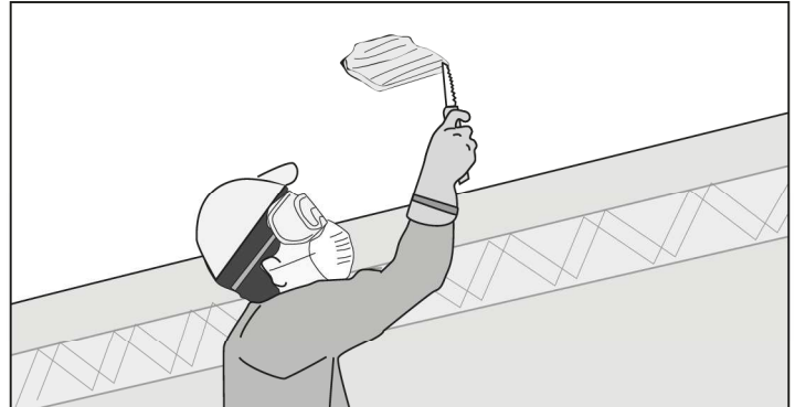
Fig.6. Enlarge the initial hole so that you can see the joist.
