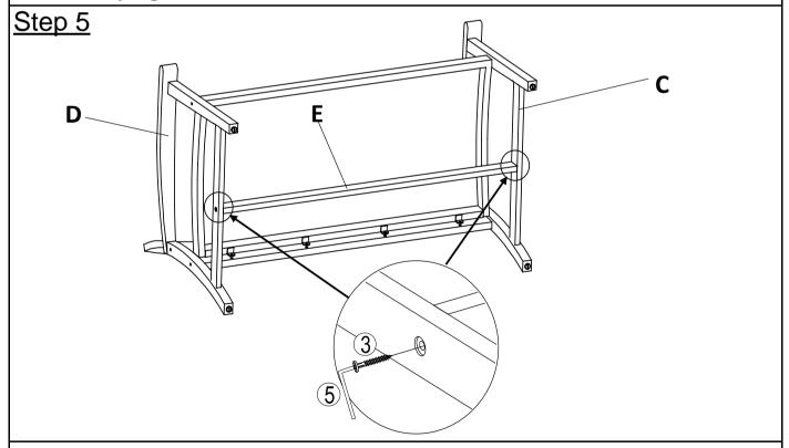
Insert Leg Support Bar (to Right Leg Panel (C) and Left Leg Panel (D) using Screw (3) with Allen key (5) as shown above.
