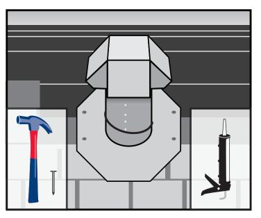
**3**. Secure octagonal flange with fasteners and caulking as approved by your local building code. Install remaining shingles in accordance with manufacturer's specification
