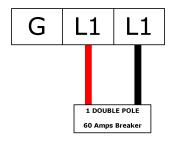
Check all wires to make sure they are securely fasten and tight. Before turning the power ON make sure the system has been flushed as required in the plumbing section. When the unit is powered up turn the control knob to turn ON the GREEN LED indicator light. You can set or adjust your temperature at any time between 80°F - 125°F (26° - 51°).
