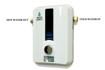
Once both water lines are fastened and secured you MUST run water through the unit for at least 2 minutes to FLUSH any air pockets (purging) in the lines, it is recommended that all faucets, showers etc be run. Failure to follow this step can cause permanent damage to the unit. This procedure MUST be performed before any electrical power is turned on.
