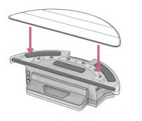
2. Open the tab and fill the reservoir with water.
