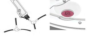
4. Clean the main brush and all its components, including the brush gate and brush compartment.
