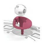
3. Clean the wheel and all its components, including the assembly and wheel socket.
