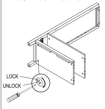
Wood dowel Cam lock bolt Cam lock Small head Large head
