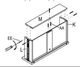
c) Tighten panels (K) and (L) to panel (J) with screw (EE). Join support bar (0) to panel (J) with dowel (AA).
