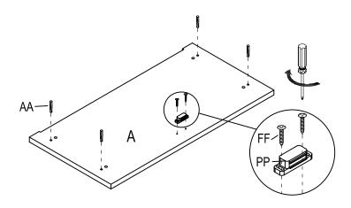
b) Join panel (A) to the assembled body with dowel (AA).
