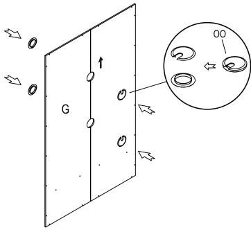
b) Tighten panel (G) to the assembled body with screws (FF) as shown.
