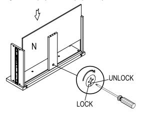
b) Insert lock (CC) into support bar (0).
