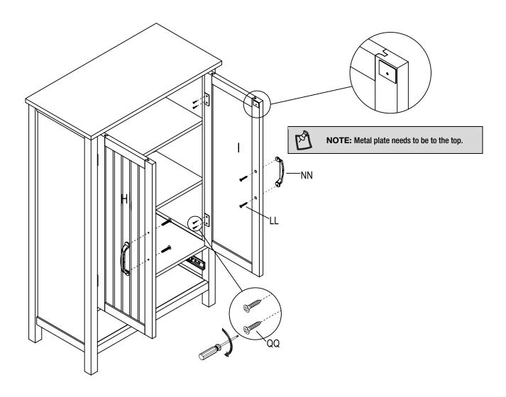
□ b) Attach handle (NN) to doors (H) and (I) with the handle bolt (LL).
