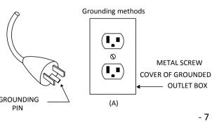
This appliance is designed to use on a nominal 120V circuit, and has a grounding plug that looks like the plug illustrated in Figure (A).
