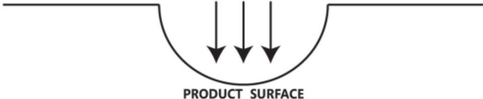
A THIN LAYER OF KLEEN KOTE FILLS IN THE MICRO POWRES, PREVENTING STICKAGE
