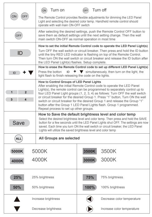
Power OFF the LED Panel Light and then power it ON. The last saved brightness (which is saved by the button "SAVE") and the last saved color temperature (which is saved by the button "SAVE" or "OFF") will be displayed by default. The defau factory setting of the light is 100% brightness and 4000K.
