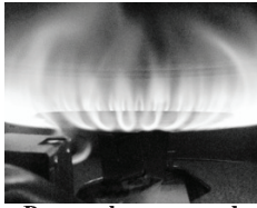
Proper burner and pilot burner pattern.
