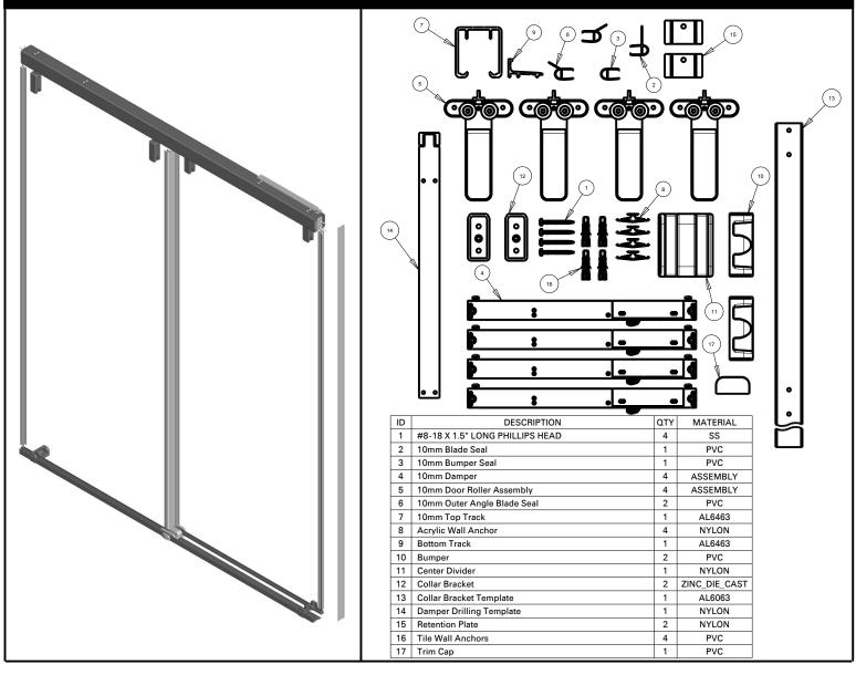
MATERIAL: Anodized Aluminum Extrusions (Track) and Zinc Die Cast (Mounting Brackets).
