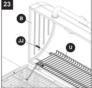
24. Fully tighten M6x30 bolts (JJ) on each side of lid and firebox assembly (B).
