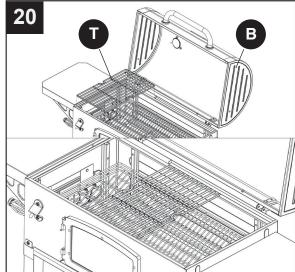
21. Place a second grate (T) on the lower grate frame of the lid and firebox assembly (B) (far left side). Place the third grate (T) on the upper grate frame of the lid and firebox assembly (B) as shown.
