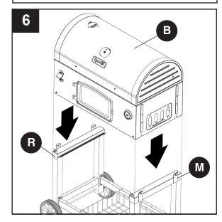
7. Secure lid and firebox assembly (B) on top of left leg assembly (R) and right leg assembly (M) using six M6x20bolts (BB).
