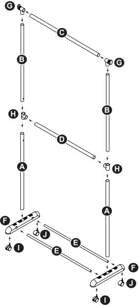
STEP 2: Firmly insert bottom vertical tubes (A) into the base, make sure the pinholes are on top and facing each other.
