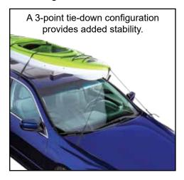
Straps may wear paint at contact points. To prevent damage, make sure contact points are clean and padded with a strap protector or soft cloth.
