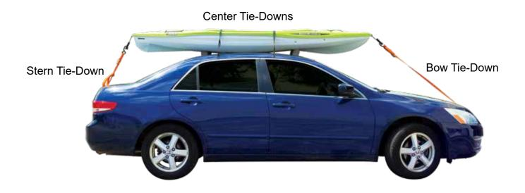
Center Tie-Downs: Loop the black cam buckle straps around the center area of the kayak and the vehicle roof, looping them through the open vehicle doors. Tighten each strap securely.
