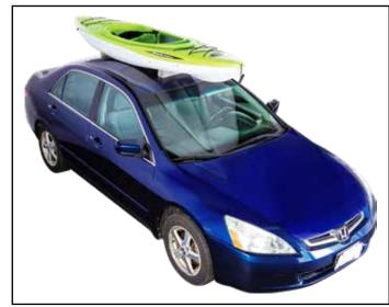
**Always** tie down the **front and rear** of the kayak. The included tie-down ropes or cam buckle straps may be used. Attach the tie-downs to a secure, metal tie-down point on the vehicle, such as a tow loop, frame hole, or metal bumper, and a secure point on the kayak, such as a grab handle. Make sure the front and rear tie-downs have even pressure. Be careful to not overtighten.
