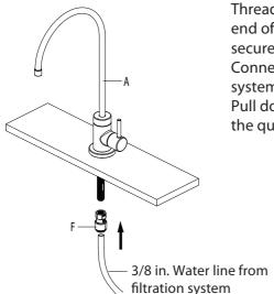
Thread the quick connect adaptor (F) onto the end of the faucet assembly (A) stud, and tighten securely using a wrench.
