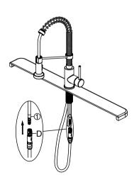
Push the quick connector (D) firmly upward and attach it to the receiving block (1). Pull down moderately to ensure the connection has been made.
