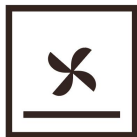
Fan and bottom heater on
