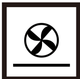
Circular Heater Fan with bottom element
