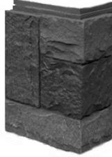
**Random Rock Outside Corner** - 4pcs. Per carton (2 left, 2 right). 11" x 15 ½" (Long side) and 7" x 15 ½"( short side) Used to wrap 90° corners and sit flush to Random Rock Panels preventing compound miter cuts and caulking of the joints.
