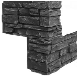
**Stacked Stone Corner** - 4pcs. per carton (2 left, 2 right). 13¾" x 12" (long side) and 4 ¼" x 12" (short side). Used to wrap 90° corners and sit flush to Stacked Stone Panels preventing compound miter cuts and caulking of the joints.
