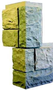
**Slatestone Outside Corner** - 4pcs. per carton (2 left, 2 right). 12¾" x 8¼" (long side) and 4 ¼" x 8 ¼" (short side). Used to wrap 90° corners and sit flush to Slatestone Panels preventing compound miter cuts and caulking of the joints.
