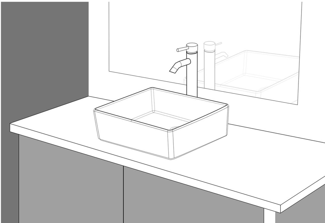
**Step#2:** Once the position is confirmed, mark the center of the drain hole and set aside the vessel sink. Draw a 3 inch diameter circle around the center of the drain hole. Use a jigsaw or a power tool to cut the opening on the countertop.
