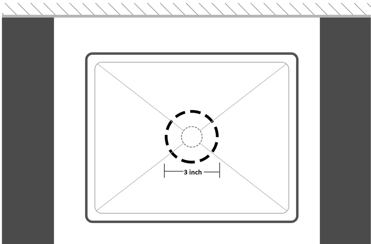
**Step#3:** Install drain according to manufacturer's installation instructions. (Note: drain not included, and do not overtighten the drain, which will damage the sink surrounding area.)
