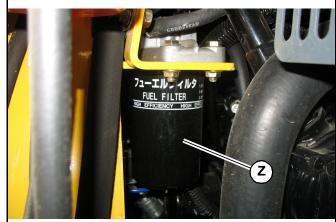
Fig. 142 - Engine Fuel Filter
