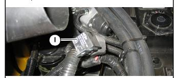
Fig. 172 - Engine Pre-heat Relay
