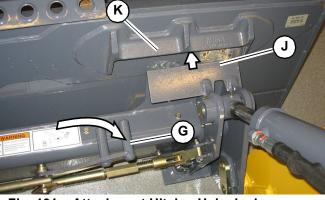
Fig. 101 - Attachment Hitch - Unlocked
