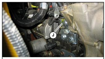
Fig. 166 - RT250 Engine Start Relay
