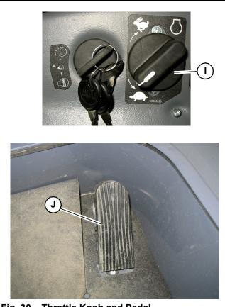
Fig. 30 - Throttle Knob and Pedal
