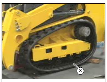
Fig. 154 - Track Installed Before Tensioning
