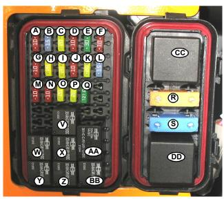
Fig. 168 - Fuses - Engine Compartment
