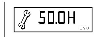
Fig. 123 - Maintenance Required Screen
