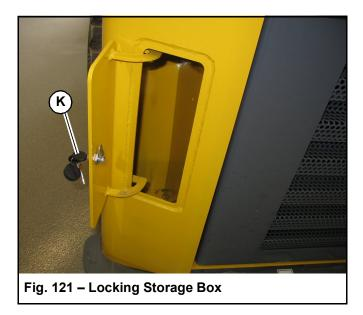
Use the accessory key (supplied with the ignition key) to lock/unlock the storage box.
