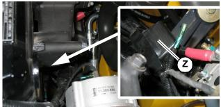
Fig. 173 - Fuses - Power-A-Tach®, Pre-Heat
