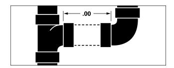
Cut pipe to required length, making sure cut is square. (See page 10 for a listing of proper tools.)
