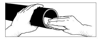
Clean all dirt, moisture, and grease from pipe and fitting socket, using a clean, dry cloth.
