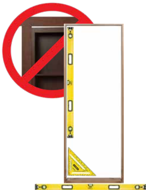
Move lower jamb out half pop distance.
