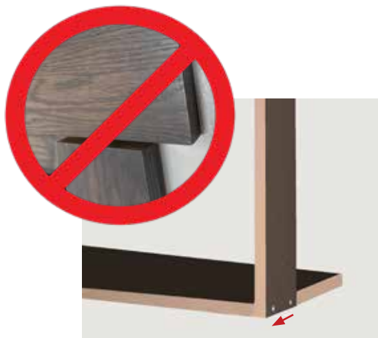
Move lower jamb out half pop distance.
