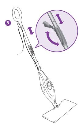
5 For your comfort, you can adjust the height of the mop. Just lift the latch on the tube 90 degrees to the open position. Holding the handle, extend the tube to the height that's right for you and then close latch to locked position.
