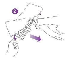
important: Always make sure the mop is unpluged from the wall when not in use. Never fill the mop, attach the mop head, change or remove the microfiber pocket when the mop is plugged into the wall. To prolong the life of your Shark® Pro Steam Pocket® Mop, we recommend using distilled water. Make sure you only add water to the tank. Chemicals or cleaning solution may damage the appliance and could be unsafe for you and your family.
