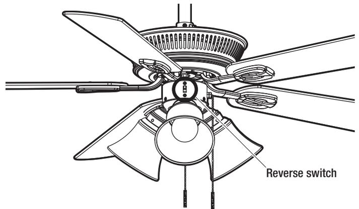
**Warm weather - (Counterclockwise Direction)** A downward air flow creates a cooling effect. This allows you to set your air conditioner on a warmer setting without affecting your comfort.
