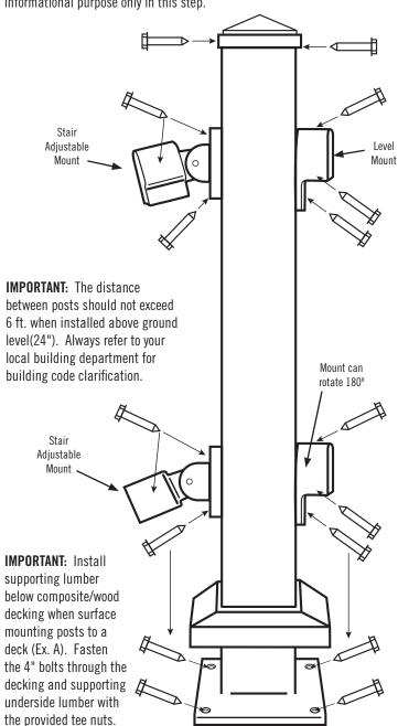
Note: When installing the post base into ACQ lumber, use stainless steel bolts (not included)
