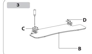
Screw up the six screws through the steel plate to the back of the keyboard tray
