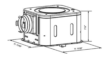
Listed for use in insulated ceilings (Type I.C.) Do not install directly over tub/shower
