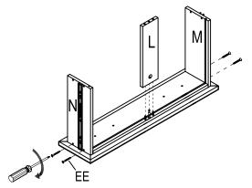
d) Slide panel (0) into the grooves on panels (M) and (N).
