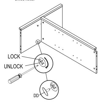
$\Box$  e) Cover the cam holes with the cover (DD).
