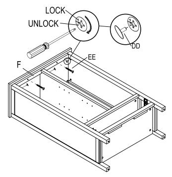
e) Cover the cam holes with the cover (DD).
