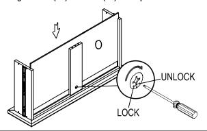
e) Tighten panel (P) to the assembled body with screw (EE) and dowel (AA).
