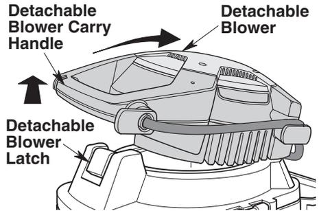
2. To replace the detachable blower onto the lid assembly, position detachable blower above the indented area of the lid assembly. Rotate the detachable blower down until the travel of the unit stops.
