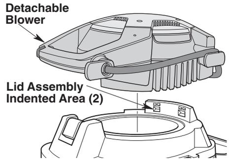
3. Lightly press down on the carry handle of the detachable blower until you hear the “snap” of the detachable blower latch engaging the detachable blower. The detachable blower is now latched to the lid assembly.
