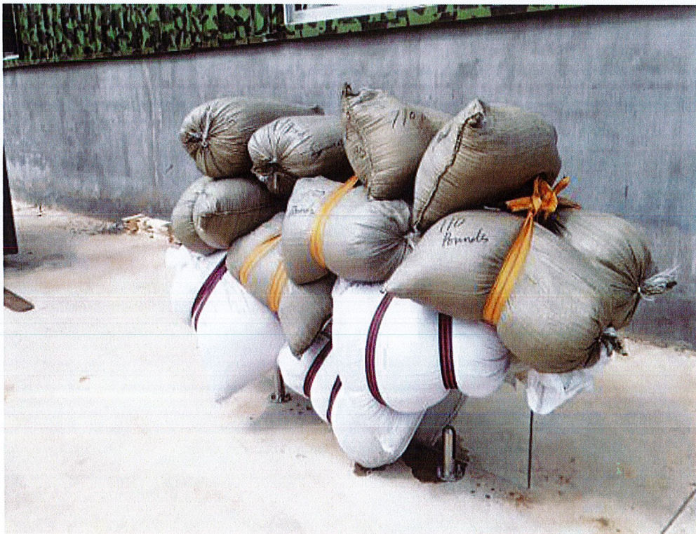
Photo 1: Panel loaded vertically with 2,520 pounds.
