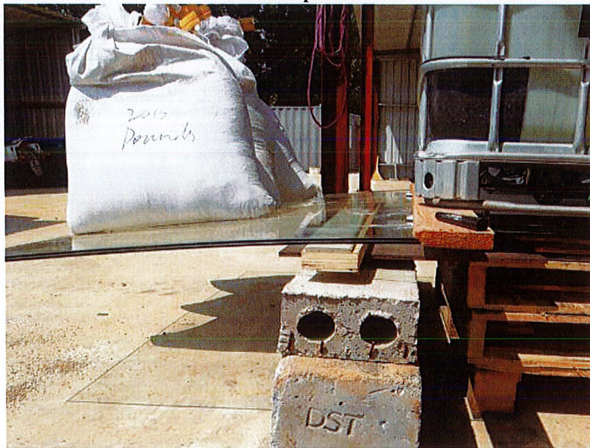
Diagram 1: Test rig lying on its side, looking from above, showing panel supported at 28" and at bottom of panel
