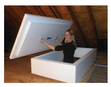
The Energy Guardian® R-20 Pull-Down Ladder Cover insulates and seals attic pull down ladders of virtually all sizes while providing easy access to the attic for the homeowner. The unit is installed in the attic and creates a cavity for the ladder to fold into when the ladder is not in use. When assembled, the kit has the following outside dimensions: 14.75" H x 33" W x 61" L (inside dimension are 10" H x 27" W x 55" L).
