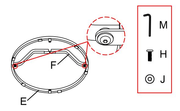
**Step 6**: Attach support bar G to base E with 2pcs bolts H and 2pcs washers J,using Allen wrench M. Note:Don't fully tighten all the bolts.
