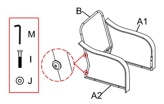
**Step 3**: Attach seat C to arms A1&A2 with 4pcs bolts I and 4pcs washers J,using Allen wrench M. Note:Don't fully tighten all the bolts.
