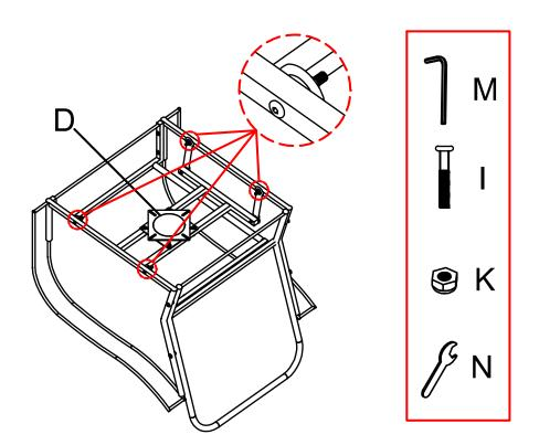
**Step 8**:Attach the assembled base E to U-Shape Fitting D with 4pcs bolts I ,8pcs washers J,4pcs spring washers L and 4pcs nuts K,using Allen wrench M and wrench N. Note: Please fully tighten all the bolts.
