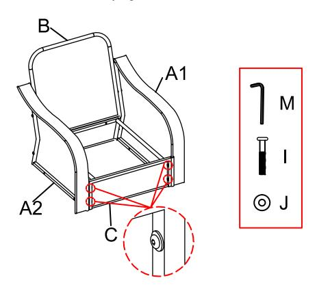
**Step 4**: Attach seat C to back B with 2pcs bolts I and 2pcs washers J ,using Allen wrench M.Note:Don't fully tighten all the bolts.
