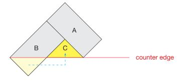
Always push part C up against A and B. Any gap that remains at the bottom countertop can be caulked later.
