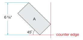
Mark a tile using your Speed Square and pencil, drawing a cut-line from one corner at 45°. Using the chop saw (miter box) cut the tile on the marked line.
