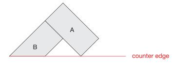
Fill in the remaining triangular area with the cut corner (C).
