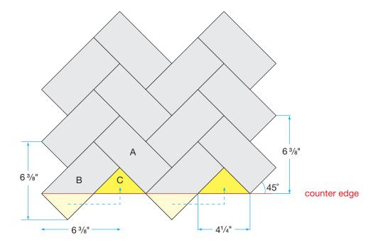
For each vertical edge (left and right sides), fill open spaces with cut corners (C) or measure and cut custom pieces as needed.
