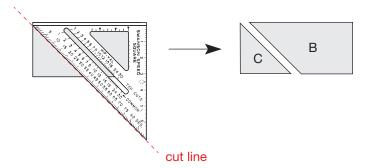
**Note:** Depending on the miter saw you're using, you may need to compensate for the saw's blade width. We recommend you "cut out" the cut-line, (center of saw blade cuts center of cut-line) instead of cutting on either side of the line as usual. Any gap should be left on the bottom or side terminations when applying cut tile parts B and C.
