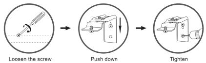
a-9 Loosen the furthest screw on the extended part of the bracket.
