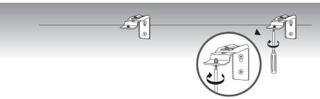
Loosen the screw one turn
