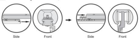
a-12 Remove the red pin that holds the slider together (can be reused to assist with the rest of the installation.)
