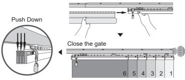
2-4 Push the tab on the end cap up to unlock, remove the end cap, and insert the panel's rubber liner into the weight
