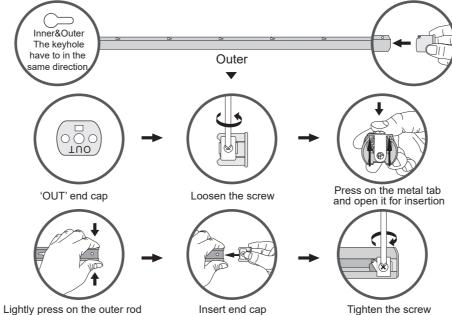
a-4 Install the outer track segment with the end cap. (See Note 4 for recommended bracket positions.
