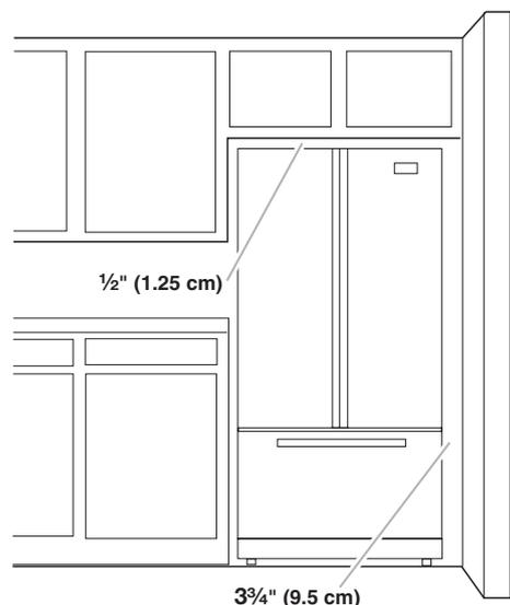
To ensure proper ventilation for your refrigerator, allow for a 1/2" (1.25 cm) of space on each side and at the top. Allow for a 1" (2.54 cm) space behind the refrigerator. If your refrigerator has an ice maker, allow extra space at the back for the water line connections. When installing your refrigerator next to a fixed wall, leave a 3<sup>3</sup>/<sub>4</sub>" (9.5 cm) minimum space between the refrigerator and wall to allow the door to swing open.
