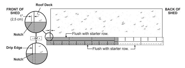
Install second row of shingles flush at top of first row's rain slots. Ensure 1" overhang or flush to drip edge at front, stagger each row.
