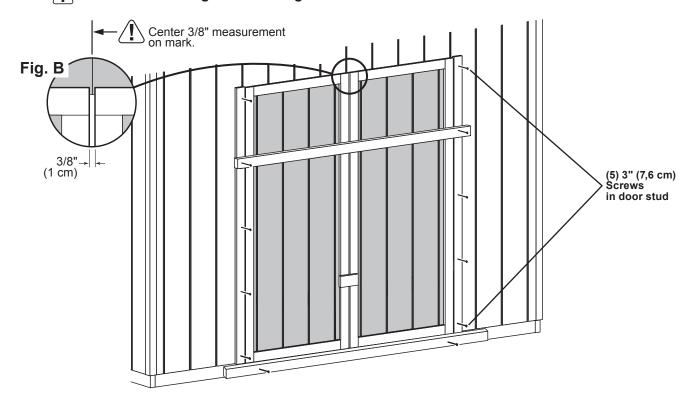
Remove temporary supports and check to make sure doors open and close properly.
