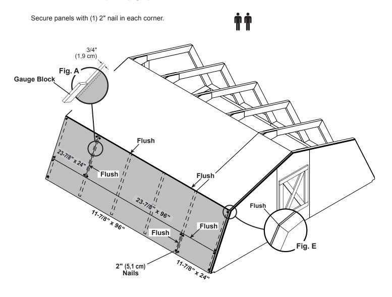
7 Install 11-7/8" x 96" and 11-7/8" x 24" roof panels flush to the installed panels. Secure panels with (1) 2" nail in each corner.
