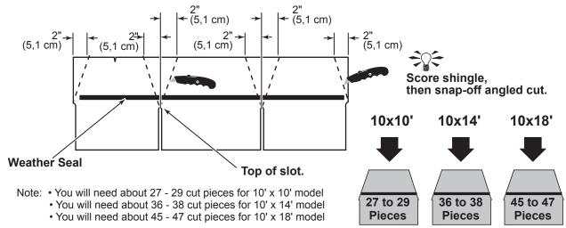
Install first ridge cap flush to shingles at front, as shown.
