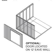
Nail lower edge of panels to floor with 2" nails spaced 6" apart.
