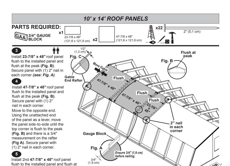
Move gable end rafter edge until it is 1/2" from the 23-7/8" x 48" roof panel
