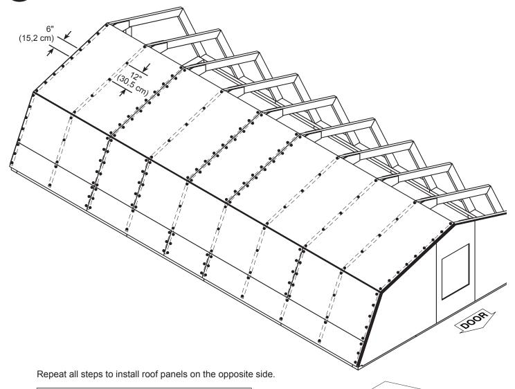
We suggest installing the 2nd set of panels in the configuration shown (Fig. F). Install the 96" panels first.
