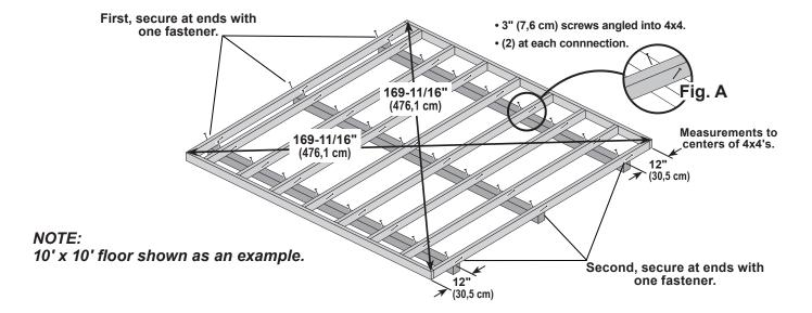
4x4 runners are generally installed 12" (30,5 cm) from ends of floor frame and under any seams.
