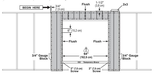
Install 48" x 84" and 23-7/8" x 84" panels flush to installed panels and 1-1/2" from the top plate. Secure panels with 2" nails spaced 6" apart on edges and 12" inside panel.
