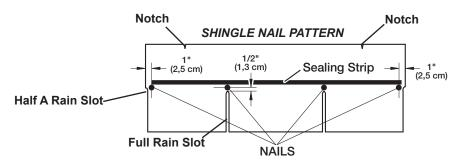
/!\ NEVER DRIVE FASTENERS INTO OR ABOVE SEALING STRIPS.
