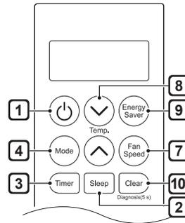
**Cool** - This mode is ideal on hot days to cool and dehumidify the room quickly. Use the **Temp**  $\wedge$   $\vee$  buttons to set the desired room temperature and use the **Fan Speed** button to set the desired fan circulation speed.
