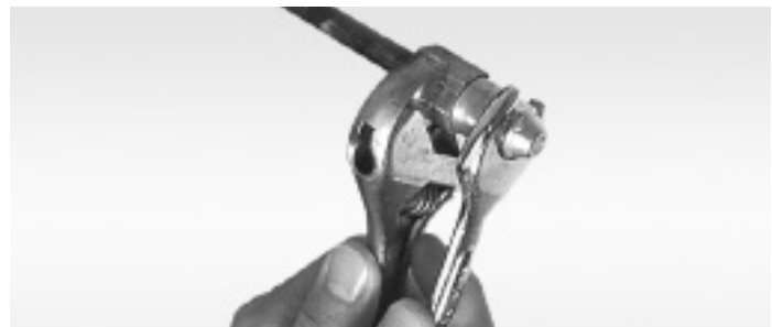
Figure 7 Carefully support the nozzle adapter when removing or installing nozzle
