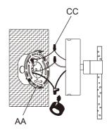
4. Place fixture body (A) onto the mounting plate (AA), securing with previously removed flat head screws (DD).
