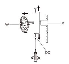
2. Attach mounting plate (AA) to outlet box (not included) using outlet box screws (BB).
