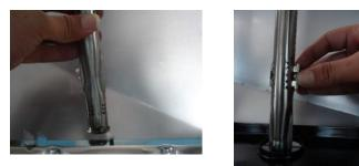
**Step 3.** Secure the main burner on the back wall of fire box with "R" Pin.
