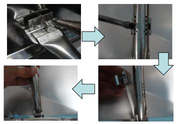
**Step 2.** Insert the burner onto the orifice and secure the burner pin cover on the burner, as shown below, make sure burner hole aim at orifice .
