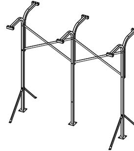
B) For double-sided units, attach (2) Knee Braces to the first Upright and then every other Upright with 3/8" x 3" bolts, 3/8" washers, 3/8" lock washers, and 3/8" nuts. Anchor each Knee Brace by drilling a 3/8" hole and fastening with a wedge anchor.
