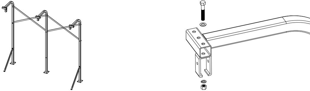
Fasten the Channel Supports to the uprights with ½" x 3" bolts, ½" washers, ½" lock washers, and ½" nuts.
