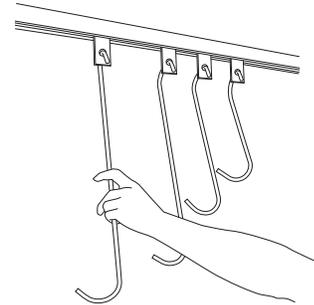
Insert the hooks through the holes in the tabs that are hanging down from the Trolleys. Each hook length should be at least 3" different than the neighboring hook.
