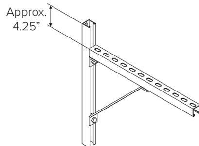
Mount the remaining 24" Slotted Tracks horizontally and protruding from the wall so that the slotted surface of the Slotted Track is 4.25" below the top edge of the vertical 24" Slotted Track. Use the Knee Braces, Angle Brackets, and the Spring-loaded Nuts and Hex Head Cap Screws to secure the horizontal Slotted Track in place.
