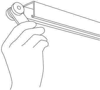
Insert the Trolleys into the open end of the 96" Slotted Track.
