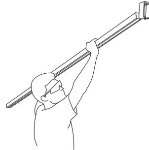
Slide 96" Slotted Track through the Channel Trolley Supports so that the centers of the brackets are 2 feet from the end of the Slotted Track.
