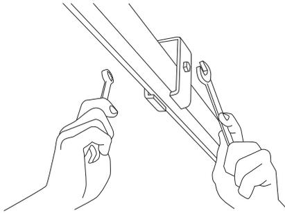
Secure the Channel Trolley Supports onto the 96" Slotted Track by tightening the Hex Head Cap Screws and Flange Nuts through the holes in the Channel Trolley Supports.
