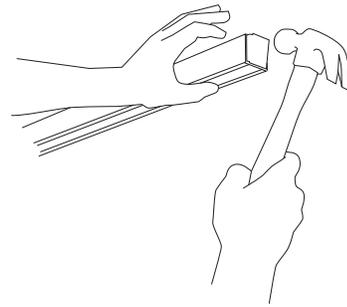
Hammer an End Cap into one end of the 96" Slotted Track.
