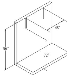
Mount 24" Slotted Tracks vertically to the wall with the appropriate anchors. Use a level for greatest accuracy. The bottom edge of the Slotted Track should be approximately 72" off the floor. The Slotted Tracks should be 4' apart from each other, and the end Slotted Tracks should be 2' from the eventual position of the end of the Trolley track.
