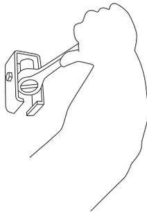
Mount Channel Trolley Supports in ceiling with appropriate anchors so that the centers of the brackets are 2 feet from each end of the 96" Slotted Track and 4 feet apart from each other.
