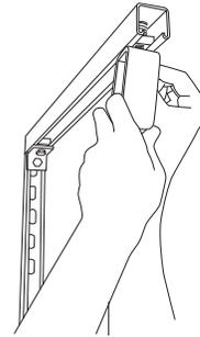
Attach the Track Rack to the Wall Mount assemblies by securing the Channel Trolley Supports to the horizontal 24" Slotted Track with the remaining Spring-loaded Nut and Hex Head Cap Screw. The edge of the Slotted Track Mounting Bracket should be flush with the edge of the 24" Slotted Track.
