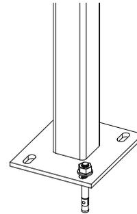
Anchor each Upright by drilling 3/8" holes and fastening with wedge anchors.
