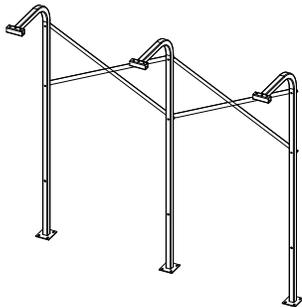
A) For single-sided units, fasten the Upright Braces to the Uprights with 3/8" x 3" bolts, 3/8" washers, 3/8" lock washers, and 3/8" nuts.
