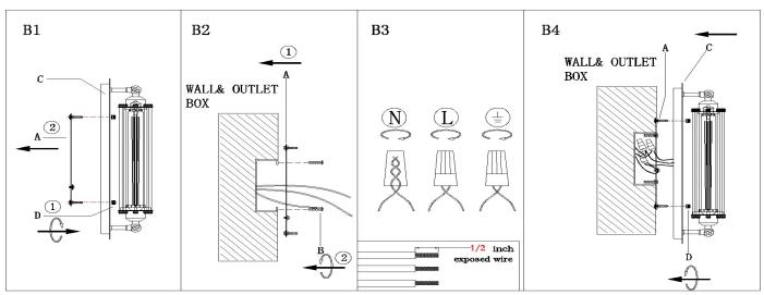
Step B1:Unscrew ball nuts (D)from the back plate(C) then remove the moungting plate(A) Step B2: Attach the mounting plate(A) to outlet box with the mounting screws(D) Step B3: Make wire connections
