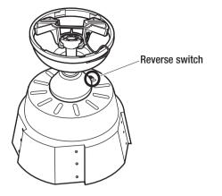
Cool weather - (Clockwise Direction) An upward air flow moves warm air off the ceiling. This allows you to set your heating unit on a cooler setting without affecting your comfort.
