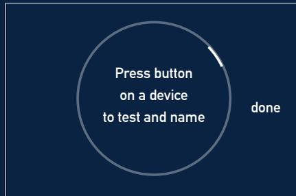
When the Keypad prompts you, remove the battery tab on the device you want to install, then press its Test Button.
