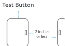
The diagram shows a square sensor on the left and a rectangular magnet on the right. A vertical dotted line points to the top of the sensor, labeled "Test Button". A horizontal dotted line between the two pieces is labeled "2 inches or less".
