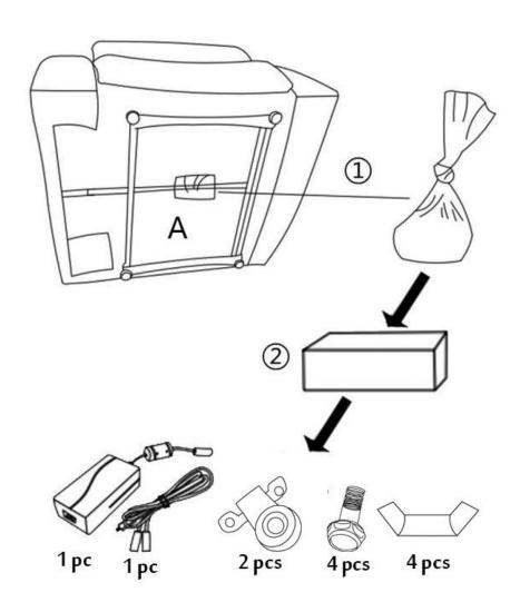
Place the main seat (A) on it's back, and fixing the two universal wheel with bolts as below:
