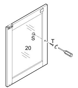
Attach handles (S) to doors (19,20) using screws (T). Tighten screws (T) with a screwdriver.
