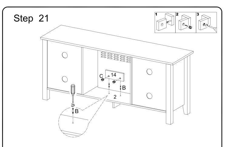
For security, insert the cam bolts (B) and use cam lock (C) to assemble the support panel (14) to the bottom panel (2).
