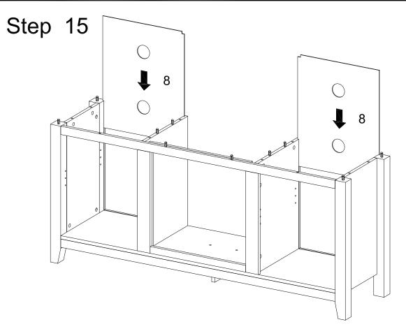
Right up the stand and slot in the back panel (8) to the side panels. Please pay attention on the corner direction of the back panel.
