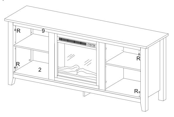
Insert plastic pivots (R) into bottom panel (2) and slat (9).
