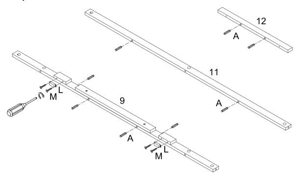
Insert the wooden dowel (A) into the front panel (9,11,12). Attach door stopper (L) to panel (9) using screws (M).
