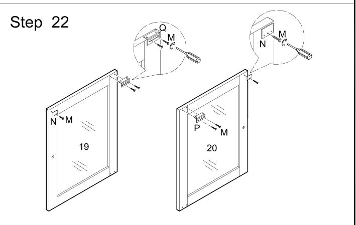
Attach door stopper plates (N) to doors (19,20) using screws (M). Attach door hinge (Q) to door (19) using screws (M). Attach door hinge (P) to door (20) using screws (M).
