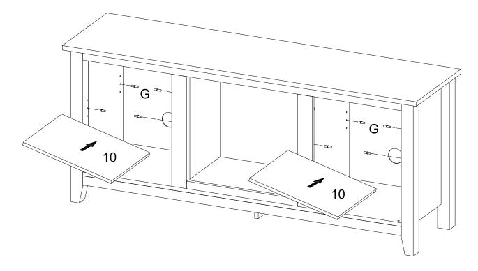
Input the shelf support pin (G) to the stand and place the wooden shelf (10) on top.
