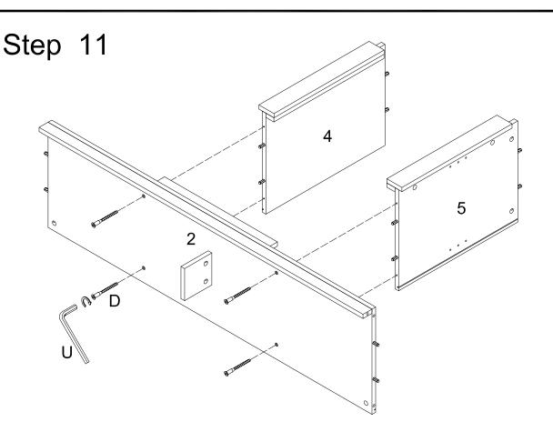
Assemble the side panel (4,5) to the bottom panel (2) and secure it by bolts (D) and wrench (U).
