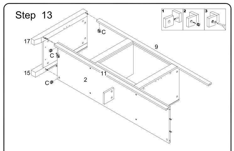
Assemble the wooden leg (15,17) to the front & bottom panel (2,9) and secure it with cam lock (C).
