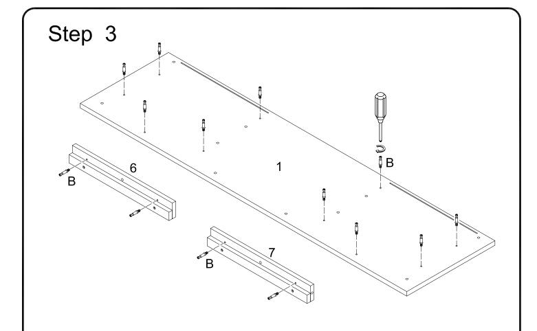
Insert the cam bolt (B) into the top panel (1) and support front panel (6,7).
