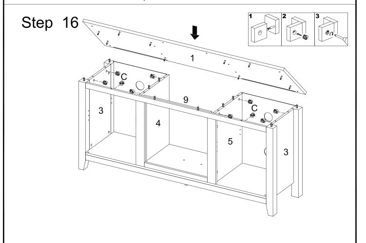
Place the top panel (1) to the stand and secure it with the cam locks (C).
