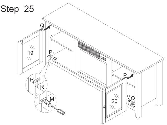
Insert door hinge (P) into bottom left bottom plastic pivot (R). Slide door (19) into place, inserting flange of door hinge (Q) into top left plastic pivot (R). Secure door hinge (P) to door (19) using screws (M). Insert door hinge (Q) into bottom right plastic pivot (R). Slide door (20) into place, inserting flange of door hinge (P) into top right plastic pivot (R). Secure door hinge (Q) to door (20) using screws (M).
