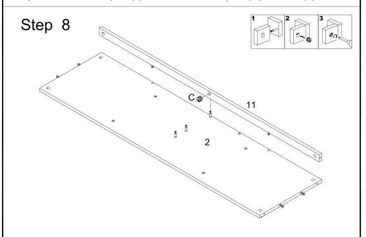
Use cam lock (C) to assemble the front panel (11) to the bottom panel (2).
