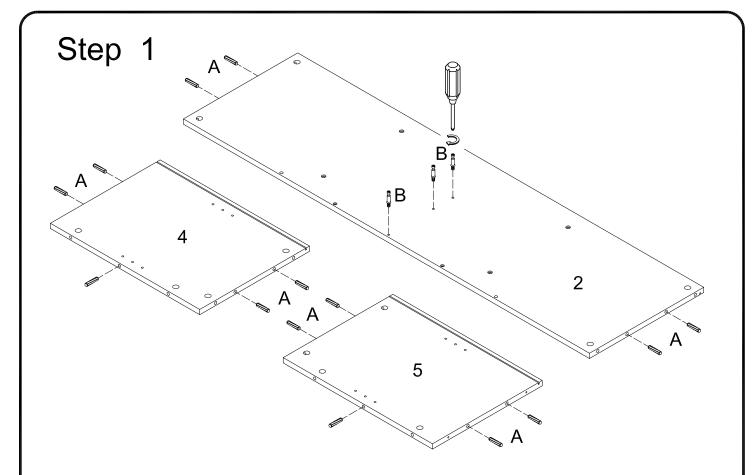
Insert the wooden dowel (A) into the bottom panel (2) and side panel (4)(5). Insert the cam bolt (B) into the bottom panel (2).
