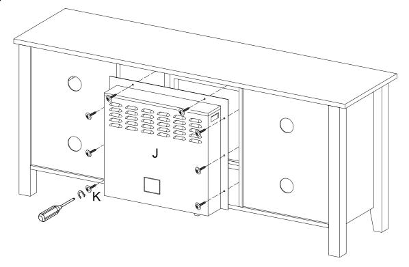
Assemble the fireplace insert (J) to the stand and secure it with screw (K).
