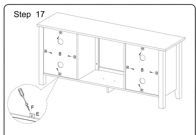
Use flat-head screw (F) and plastic wedge (E) to secure the back panel (8).
