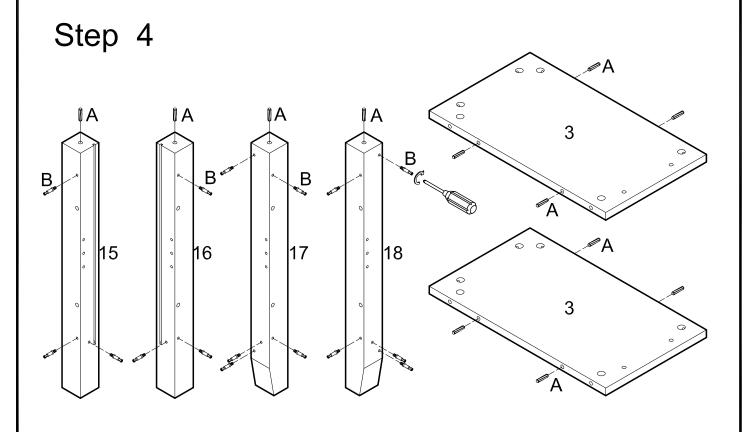
Insert the wooden dowel (A), cam bolt (B) into the wooden legs (15,16,17,18). Insert the wooden dowel (A) into the side panel (3).
