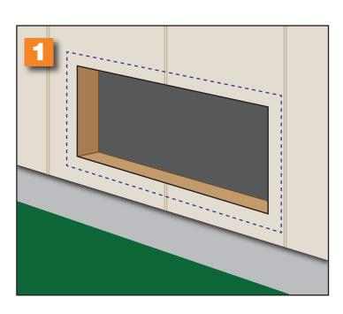
1. Remove old vent and any loose debris from opening.
