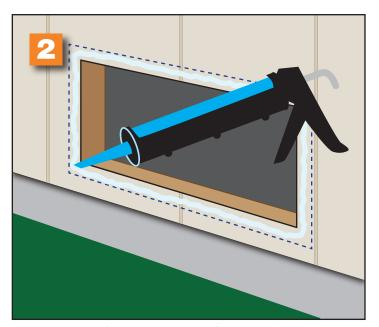
2. Apply a bead of sealant to the vent flange or wall.
