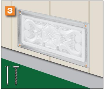
3. Using the partial punched corner fastener guides (4 per vent), fasten vent with nails or screws.
