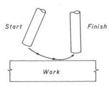
In the tapping method, the electrode is moved downward to the base metal in a vertical direction. As soon as it touches the metal it is withdrawn momentarily to form an excessively long arc, then returned to normal arc length (see figure 2).
