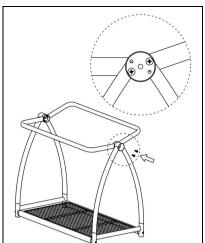
Assemble the Rail (C) to the frames using the Short Screws (F). The rail curves up toward the back.
