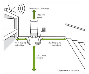
**MARNING:** To prevent the risk of your robot falling downstairs, ensure that the charging station is placed at least 4 feet (1.2 meters) away from stairs.
