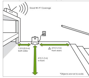
MARNING: To prevent the risk of your robot falling downstairs, ensure that the charging station is placed at least 4 feet (1.2 meters) away from stairs.
