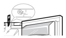
3 Hold the mouthpiece of your phone in front of the speaker that is located on the right hinge of the refrigerator door, when instructed to do so by the call center.
